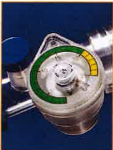
Built-in Manometer/ Measures Consistent CPAP Pressure
